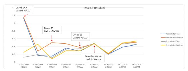
Manual grab samples were taken from the top and bottom of the reservoir at the north and south hatches. Multiple daily samples were taken within the first three days of installing the mixer. Within 90 minutes of the mixer being powered on, the reservoir had uniform chlorine residual levels of 0.30ppm. From that point forward, single samples were taken daily which indicated a uniform free chlorine residual of 0.50ppm (+/- 0.05ppm) and climbed over the subsequent ten days (Reference graph above).
